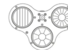
Prism 2: 3 different prisms, 6-Facet linear prism/8-facet circular prism/16-facet circular prism with variable speed and direction
