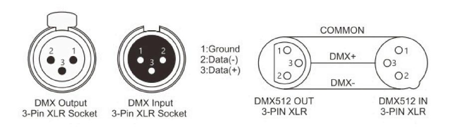
For installations where the DMX cable has to run a long distance or is in an electrically noisy environment, such as in a discotheque, it is recommended to use a DMX terminator. This helps in preventing corruption of the digital control signal by electrical noise. The DMX terminator is simply an XLR plug with a 120  $\Omega$  resistor connected between pins 2 and 3,which is then plugged into the output XLR socket of the last fixture in the chain. Please see illustrations below.
